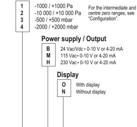
Example : CP 201-MN = pressure transmitter type CP 200, with measuring range of -1000/+1000 Pa, with power supply 115 Vac, without display.
